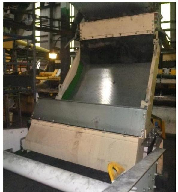
The rubber curtains and HDPE capping introduced on the sieve bend.
